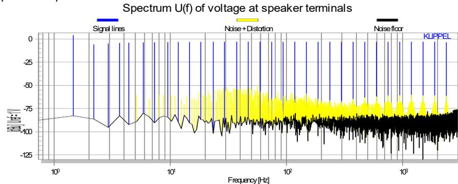
In this example the amplifier has distortion about 0,5%. They are quite good separated from the noise floor which is 20 dB lower. Whereas the distortion components fill all bins at low and medium frequencies there are clearly separated intermodulation centered around the fundamentals at higher frequencies. This kind of distortion is typical for a digital amplifier (Class D) having a poor power supply rejection.
