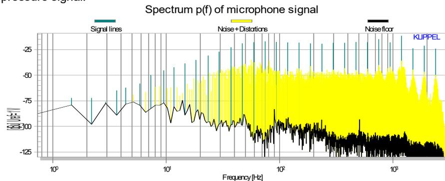
The distortion floor is almost constant up to 1 kHz. At higher frequencies the distortion are centered around the fundamental component mainly caused by intermodulation between the displacement which is a low-pass filtered signal and the current. Comparing the distortion in current and sound pressure reveals dominant force factor distortion up to 1 kHz and dominant inductance distortion at higher frequencies.
