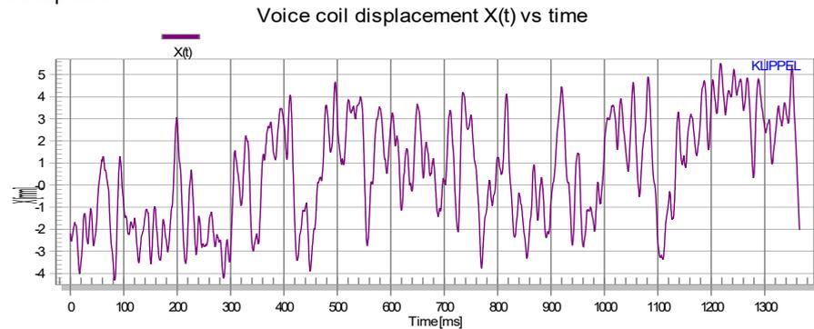
In this example the driver produced a peak to peak displacement of  $X_{pp} = 9.82$  mm. This value is also displayed on the result window **Table signal characteristics**. The time signal also reveals a good mixture of high frequency and low frequency components.
