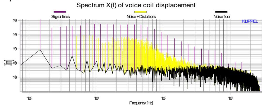
Above the resonance frequency  $f_s$  at 70 Hz the amplitude of the displacement decreases by 12 dB per octave.
