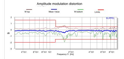
The top and bottom modulation  $M_{top}$  and  $M_{bottom}$  describe the minimal and maximal variations of the envelope of the voice tone f1. The mean modulation shows the variation in the amplitude response between the high frequency voice tone with and without the bass tone f2.
