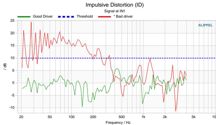
All of the golden units have some regular (peaky) distortion at 40-100 Hz which is typical for this driver. However, this regular distortion is significantly suppressed by the adaptive compensation technique. Finally a 6<sup>th</sup> driver with a hardly audible defect is measured. At low frequencies there is a clear deviation from the trained driver model indicating a defect. The effective DNR is well above 10 dB, exceeding the threshold clearly.
