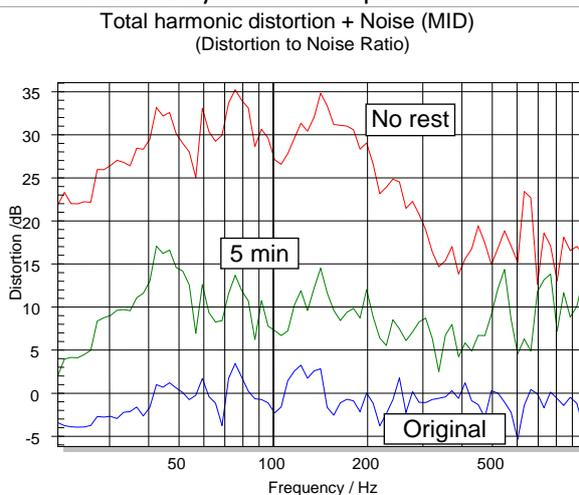
The TRF-Pro can also be used to monitor the deviation from a given nonlinear behavior. In this example a driver was subjected to a sustained elongation to one displacement limit and was released after 2 minutes. Due to the permanent stretching of the suspension the stiffness nonlinearity has changed and became softer at the rest position.
