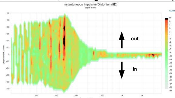
This unit is showing several clicks which appears almost randomly. This symptom can be caused by some loose particles.
