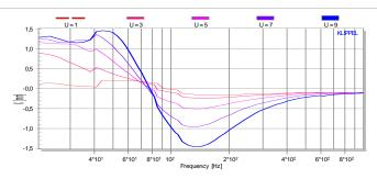
The diagram shows the response of a driver with a coil offset causing an asymmetry in the Bl(x)-curve. At frequencies below the resonance ( < 80 Hz) the coil will shifted dynamically to 1.4 mm which is the maximum of the Bl(x)-curve (self-centering capability). However, at 150 Hz the DC-displacement rises rapidly showing an instability of the motor (coil jump out effect).
