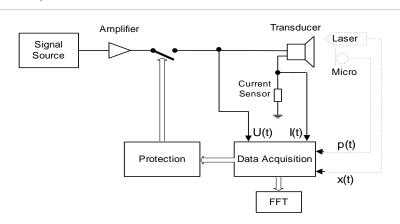
The generated excitation signal is applied to OUT 1, and may be amplified and linked via the high-power path of the analyzer unit to the transducer under test. Voltage and current sensors measure the amplifier output (at connector AMPLIFIER) and the electrical signals at the transducer terminals (at connector SPEAKER 1 or SPEAKER 2). At the beginning of the measurement the transducer is disconnected from the amplifier output to determine the amplifier gain automatically.
