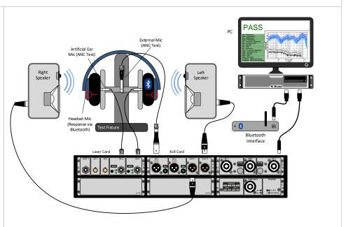
For testing audio products with complex processing algorithms like Bluetooth® enabled headsets with active noise cancelation (ANC), a transient test signal like a sinusoidal sweep (chirp) is not an optimal test stimulus. A broad-band, steady-state signal like pink or white noise is more suitable for reproducible test results of the ANC performance or
