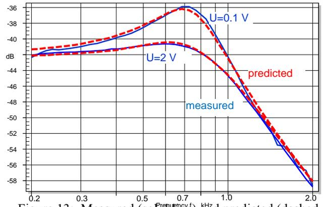
Figure 13: Measured (solid line) and predicted (dashed line) amplitude ratio of the fundamental component of voice coil displacement  $x$  and input voltage  $U$  in the small and large signal domain
