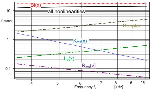
Figure 17: 2<sup>nd</sup>-order intermodulation distortion versus frequency  $f_2$  generated by a two-tone stimulus (with  $f_2 > f_1=400$  Hz) considering all nonlinearities (thick solid line) and only one selected nonlinearity in the modeling
