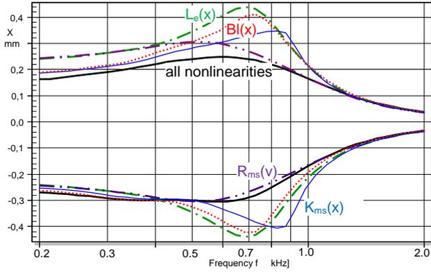
Figure 11: Peak and bottom displacement predicted by using all nonlinear parameters (solid line) and by considering each separated nonlinear cause
