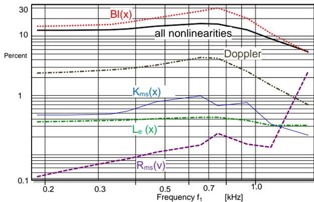
Figure 19: 2<sup>nd</sup>-order intermodulation distortion versus  $f_1$  generated by a two-tone stimulus (with  $f_1 < f_2 = 6$  kHz) considering all nonlinearities (thick solid line) and only one selected nonlinearity in the modeling
