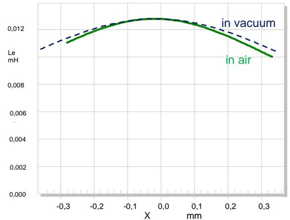
Figure 8: Nonlinear inductance  $L_e(x)$  versus displacement  $x$  of a micro-speaker measured in air (solid curve) and in vacuum (dashed curve)
