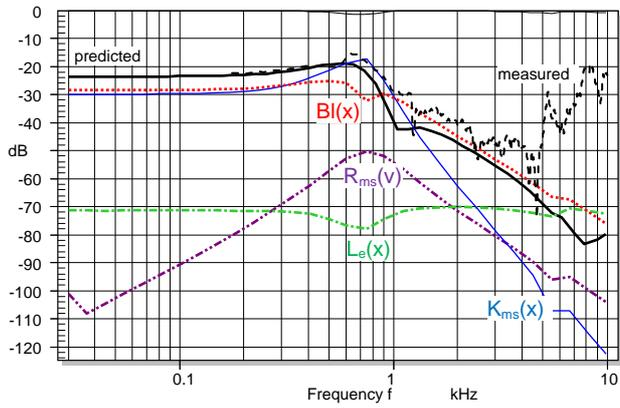
Figure 15: Measured (dashed line) and predicted (solid line) 2<sup>nd</sup>-order equivalent harmonic input distortion versus frequency  $f$  and the contribution of each nonlinearity
