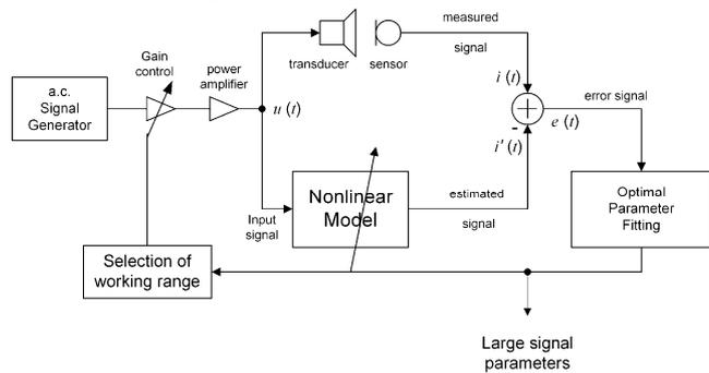
Figure 5: Dynamical measurement of transducer parameters by adaptive modeling of the input current
