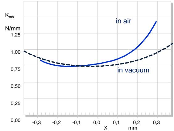
Figure 6: Nonlinear stiffness  $K_{ms}(x)$  versus displacement  $x$  of a micro-speaker measured in air (solid curve) and in vacuum (dashed curve)
