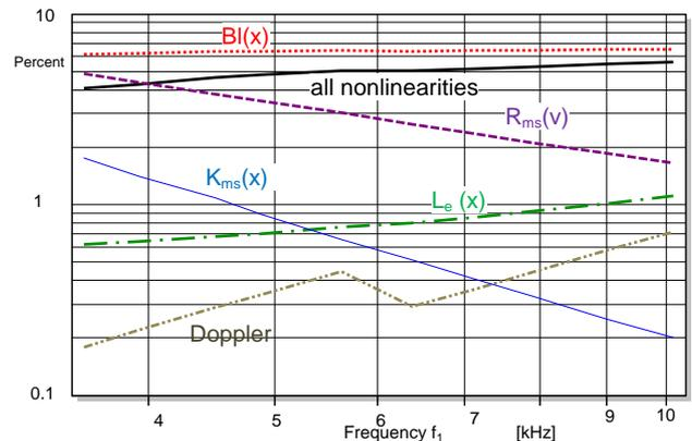
Figure 18: 3<sup>rd</sup>-order intermodulation distortion versus frequency  $f_2$  generated by a two-tone stimulus (with  $f_2 > f_1=400$  Hz) considering all nonlinearities (thick solid line) and only one selected nonlinearity in the modeling
