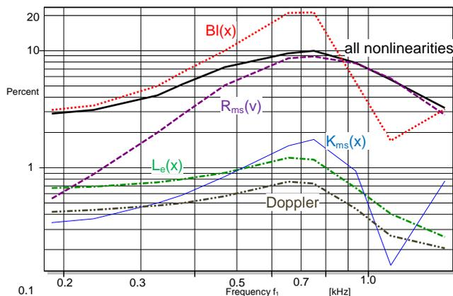
Figure 20: 3<sup>rd</sup>-order intermodulation distortion versus  $f_1$  generated by a two-tone stimulus (with  $f_1 < f_2 = 6$  kHz) considering all nonlinearities (thick solid line) and only one selected nonlinearity in the modeling
