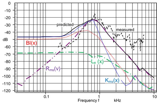
Figure 16: Measured (dashed line) and predicted (solid line) 3<sup>rd</sup>-order equivalent harmonic input distortion versus frequency  $f$  and the contribution of each nonlinearity
