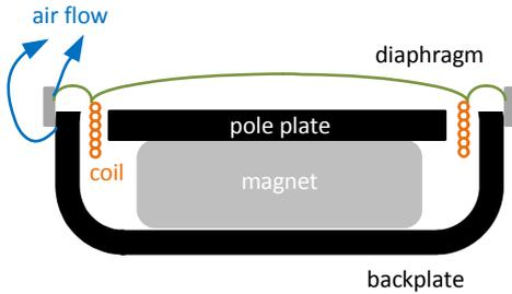
Figure 1: Sectional view of a micro-speaker
