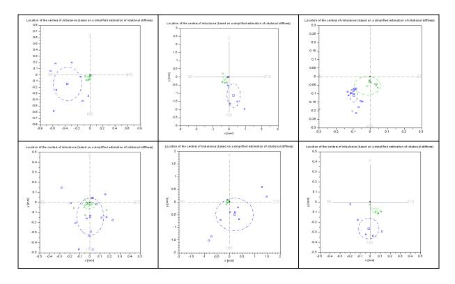
Reviewing the patterns above gives an immediate impression of the stability and spread of the production process and shows whether the problems are systematic or random. The user also gets a clear indication in which direction to search for the underlying root-cause in design or manufacturing. Repeat the measurement series after making a change to track the progress.
