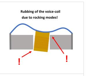
This application note demonstrates how to solve problems with rocking modes in electrodynamic loudspeaker transducers, with special attention to headphones and microspeaker drivers. Rocking modes (oscillating tilting motion of the diaphragm) at large amplitudes are highly undesired since they can cause impulsive signal distortion, limit the usable output and reduce the durability of the transducer.
