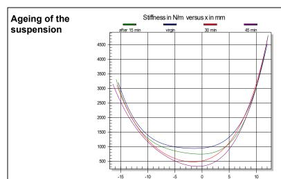
The dynamic measurement technique is also convenient for investigation of the break in and other ageing effects of the suspension. The example shows the change of the stiffness versus time while permanently exciting the spider with the audio-like test signal and performing measurements after 15 min intervals. It is interesting to see that the stiffness at higher displacements stays constant but the stiffness at the rest position.
