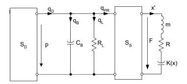
The driver generates a volume velocity  $q_D$  that divides into three parts as shown in the equivalent circuit above. The volume velocity  $q_B$  flows into the volume of the box,  $q_L$  is leaving the box through leaks and the volume velocity  $q_{PR}$  produces the force F driving the suspension part under test
