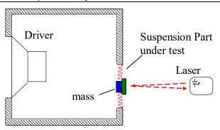
The figure above shows essential parts of the measurement setup. An 18" driver is mounted in a sealed enclosure having a second hole where the suspension part under test is placed. The outer rim of the suspension part is firmly clamped by rings.
