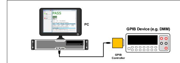
The QC External Devices task is a versatile add-on for the QC framework of the KLIPPEL Analyzer System dedicated to interfacing with arbitrary GPIB (IEEE 488) compliant measurement equipment, such as multimeters or power supplies. Simple programmable step sequences enable the user to control external devices and to include the measured data in the QC System. Full limit handling is provided to generate PASS/FAIL verdicts.
