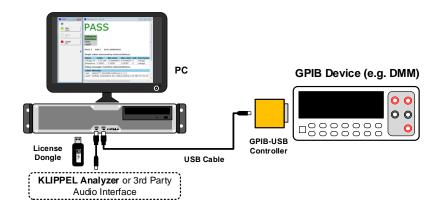
The figure above shows the minimal equipment required to use the EXD module:
