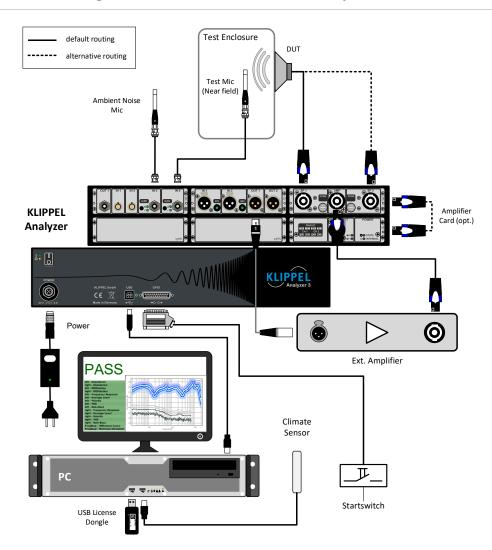
This is a typical setup for transducer end-of-line testing using QC Standard setup.
