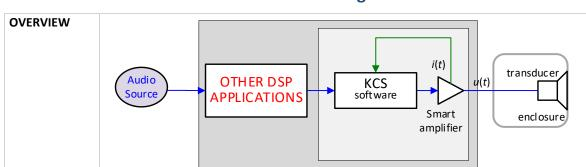
Combining the linearization, stabilization and protection capabilities of KCS with other DSP applications in the audio signal chain that are considering the electro-acoustical transducer as a (linear) black-box system offers substantial benefit. KCS enhances the performance and simplifies the system design for applications like:
