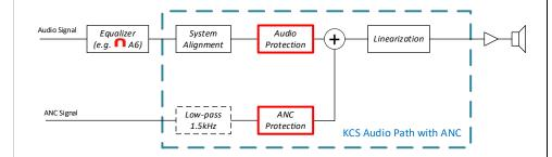
The low latency signal is provided to KCS via a separate input channel to avoid unnecessary digital filters (EQ / Alignment) adding group delay to the signal. A dedicated overload protection system for this separate input path can be applied with ultra-short latency (0.1ms) while the audio protection system has a larger, configurable latency to minimize audible artifacts.
