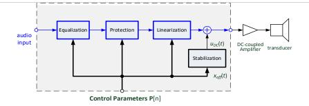
The processing of the audio input signal is performed by a feed-forward structure in the following order:
