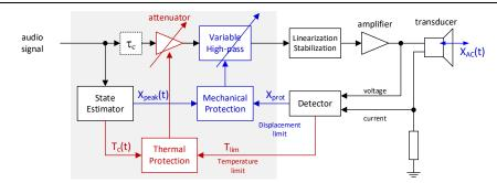
These features cannot be fulfilled by just limiting the maximal voltage or electrical input power supplied to the loudspeaker terminals. KCS generates the following state information that are related with a mechanical and thermal overload in the transducer:
