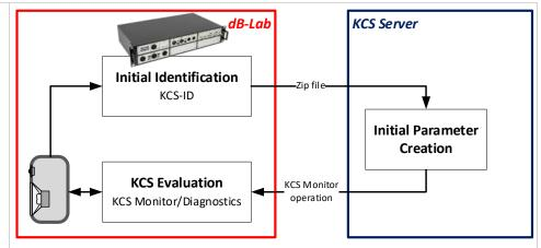
The identification of speaker parameters is done using the software module *KCS-ID Parameter Identification*. The signals recorded by the KCS-ID are sent to Klippel's *KCS Server*. This server automatically creates initial KCS data for the particular KCS hardware platform and a *KCS Monitor* operation is provided on the KCS Server's web interface. The *KCS Monitor* operation can connect to any supported KCS hardware platform and a control session can be started.
