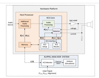
The diagram above shows a Host DSP Processor providing the audio frame for the KCS Core and additional audio processing and the KLIPPEL ANALYZER SYSTEM for operating KCS and loudspeaker diagnostics.
