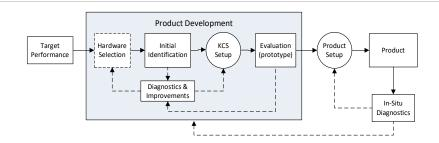
The KCS technology accelerates the development of active audio products due to the close connection between hardware and software design, simulation, measurement, diagnostics and on-line evaluation. An active loudspeaker system typically consists of a Digital Signal Processor (DSP), a power amplifier and a transducer mounted in an enclosure.
