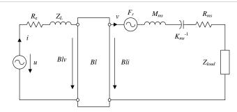
At low frequencies loudspeakers, headphones, micro-speakers and other actuators can be modeled using an equivalent network comprised of lumped elements.
