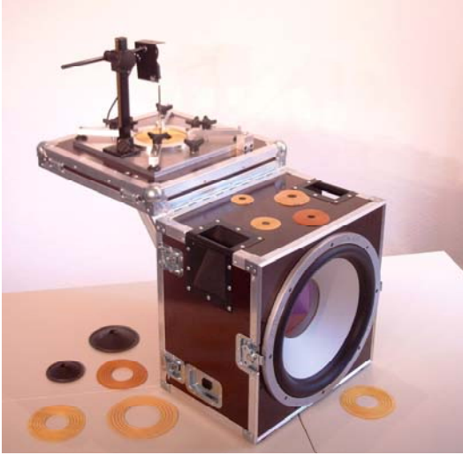
Figure 3 Open test enclosure with work bench in horizontal position
